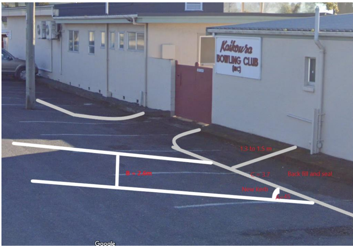
Figure 6. New kerb and footpath layout The current car parking measurements can be seen below.
