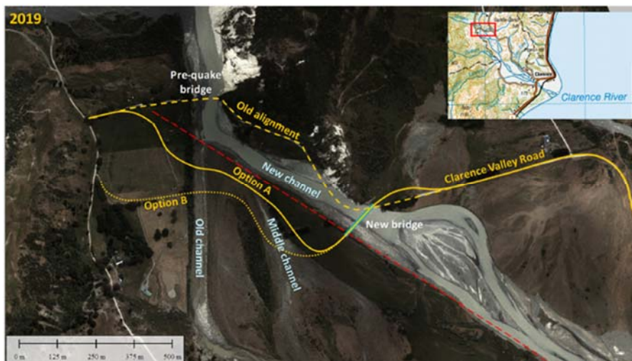
Location of a proposed new bridge downstream of Glen Alton with a ford across the old riverbed
