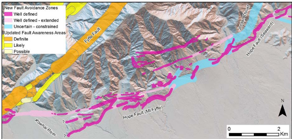
Figure A2.5 New Fault Avoidance Zones and updated Fault Awareness Areas for the Mt Fyffe Section of the Hope Fault.
