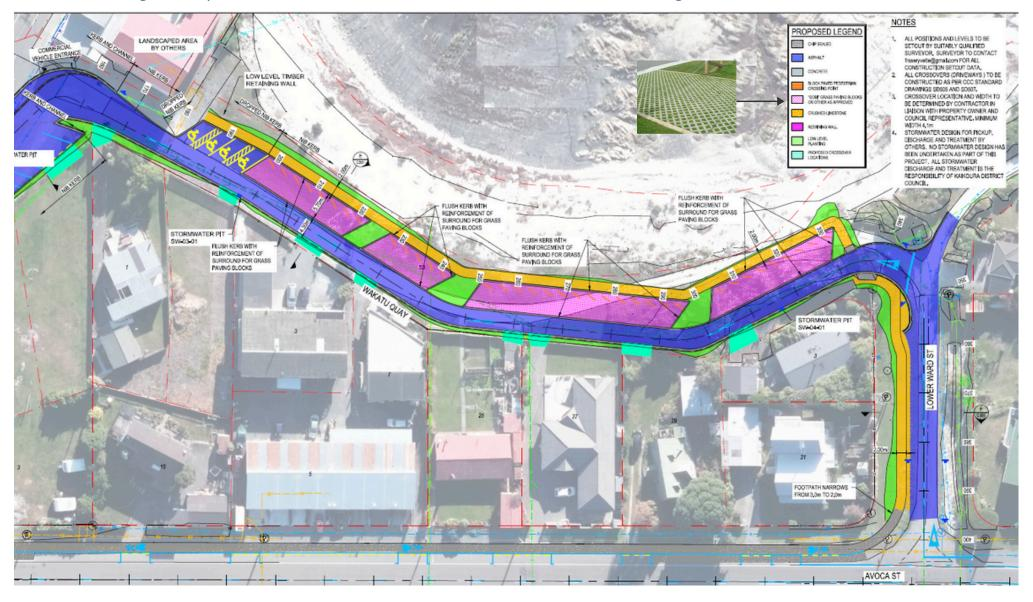
A chip seal footpath will be installed along the north side of Avoca Street along with marked parking zones.
